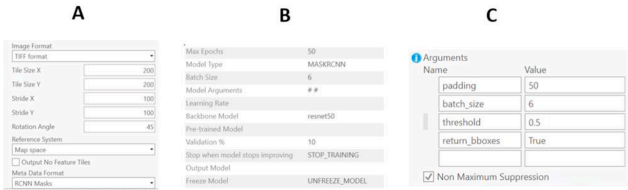
Fig. 4. Settings used for constructing and implementing a Mask R-CNN model in ArcGIS Pro. (A) Export Training Data for Deep Learning Tool. (B) Train Deep Learning Model Tool. (C) Detect Objects Using Deep Learning Tool. The padding and threshold were lowered to 10 and 0.2, respectively, for Georgetown County to ensure maximum detection of potential rings.
